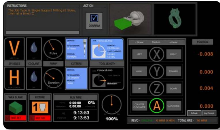
**REVO PROCEDURE MANAGER: New control software with step-by-step instructions, easy to follow graphics, and redesigned controls**
