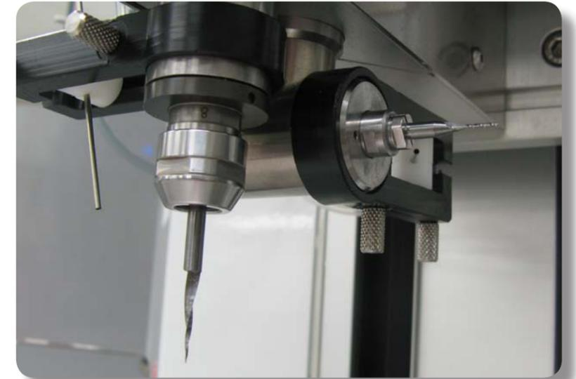
**Dual-Spindle technology produces advanced models in a single operation, virtually eliminating the need to change fixtures**
